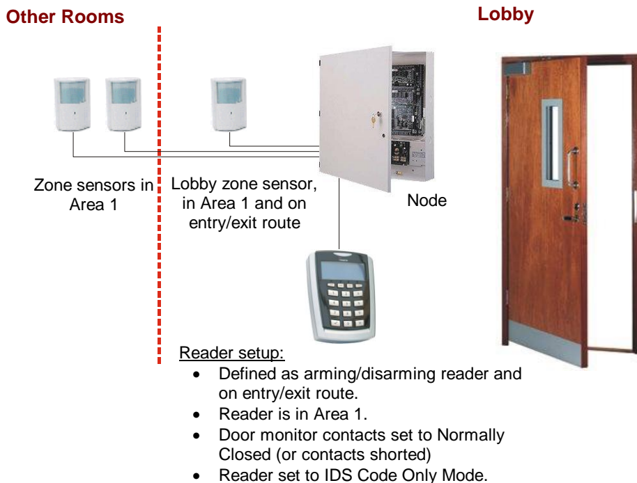
Figure 1-7: Example 3 - Internal Arming/Disarming Reader Only
